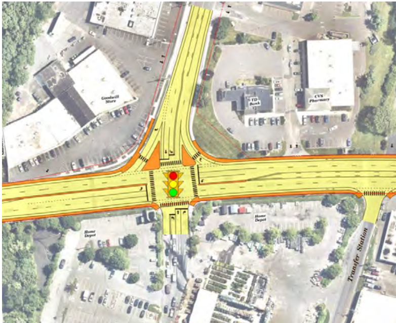
Revised Arctic Avenue signalized intersection
