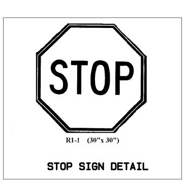
NOTE: SIGNS TO BE MOUNTED TO A GALVANIZED BREAKAWAY STEEL U POST ( BOTTOM OF SIGN SHALL BE A MINIMUM OF 5' FROM PAVEMENT )
